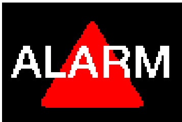
Alarms as shown in Test and Operation Mode after PIR and MW Pre-Alarm
